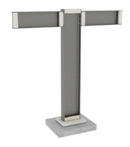
Repeate Steps 3 and 4 for the steel beam ie. install end noggings. Also install noggings at the intersection joint.
