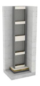
Install 200 mm width noggings at maximum 1200mm centres to coincide with the joints between the batts in Step 7. Install 100 mm width intermediate noggings at maximum 600mm centres between the 200 mm noggings as per Step 4.
