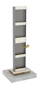
Install 200 mm width noggings at maximum 1200mm centres to coincide with the joints between the batts in Step 7. Install 100 mm width intermediate noggins at maximum 600mm centres between the 200 mm noggins as per Step 4.
