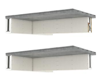
Apply extra FIREFLY Ablative Coating on all the joints / corners / edges, ensuring that there are no visible cracks or exposed green edges of the batts as seen from outside.
