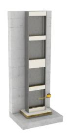
Install 200 mm width noggings at maximum 1200mm centres to coincide with the joints between the batts in Step 7. Install 100 mm width intermediate noggings at maximum 600mm centres between the 200 mm noggings as per Step 4.
