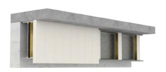
Cut a batt to a width corresponding with distance between the slab underside and bottom flange, adding 50 mm for the bottom flange overlap.
