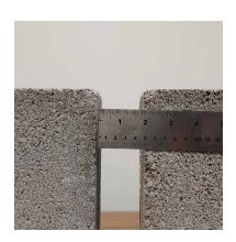
Ensure the gap is free of any dust and contaminants and relatively smooth  $% \left\{ \left( 1\right) \right\} =\left\{ \left( 1\right$
