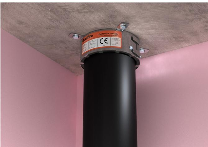
The QWR CE Marked Fire Collar must be secured to concrete and masonry construction using steel sleeve anchors.
