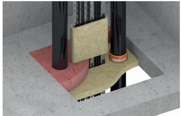
QF2 Fire Protection Compound used in conjunction with MW Mineral Wool Slab
